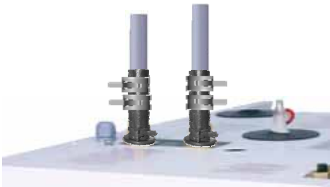
Straight Connection Components Installed
