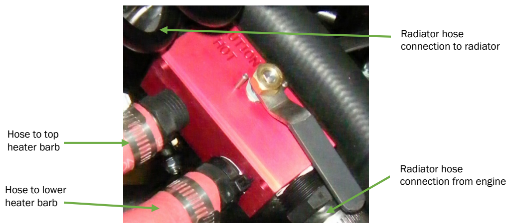
Figure 6: Installation of lengths of hose on each heater port
