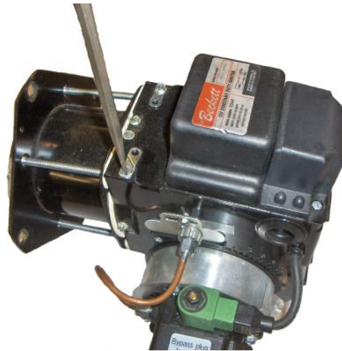
D. Using a flat head screw driver, Securely Tighten the retaining clips securing the ignition coil in place.
