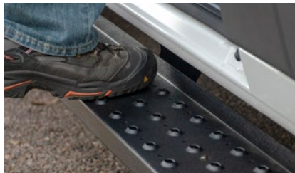
Stamped steel treads for a non-skid step that will never wear or crack
