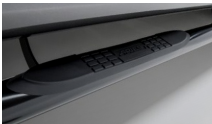
Custom, non-skid step pads for safe entry and exit
