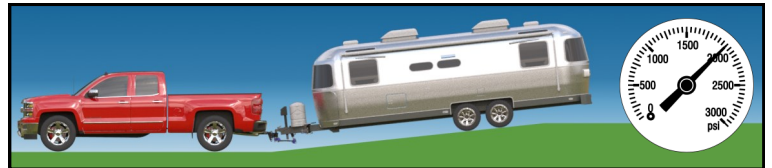
FIGURE L4: Truck and trailer angled up (higher pressure)
