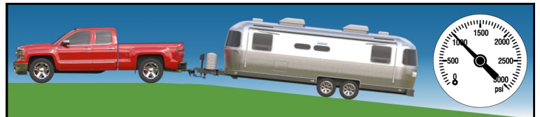
FIGURE L5: Truck and trailer angled down (lower pressure)
