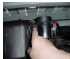
Figure C2, Step 2: Disengage the locking pin.
