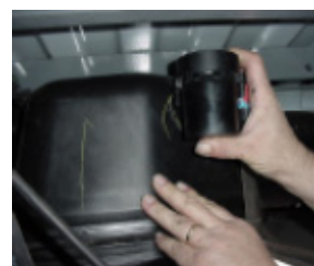
Figure C3, Step 3: Slide fuel valve from bracket.
