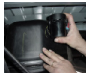
Figure C3, Step 3: Slide fuel valve from bracket.
