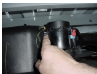
Step 2: Disengage the locking pin.
