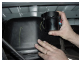
Step 3: Slide fuel valve from bracket.
