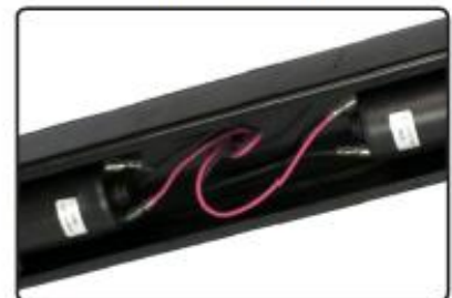
Stabilizer Jack Motor Wires
