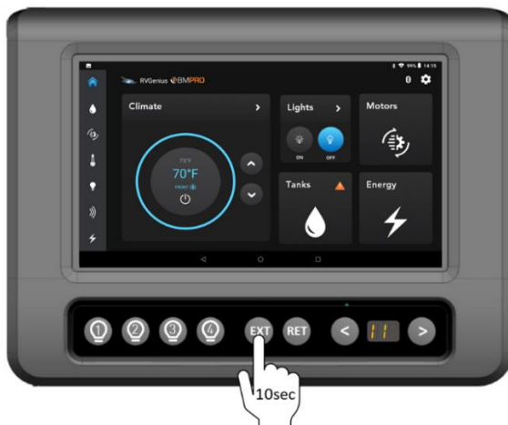
Figure 6: Go to PA, then Press and hold EXT until the number 1 scrolls across the CONTROLLER
