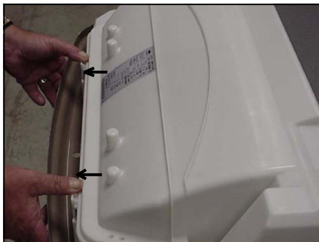
Figure 3-29 Upper Scroll Assembly Keeper Tab Release
