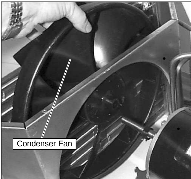
Figure 3-22 Condenser Fan Removal
