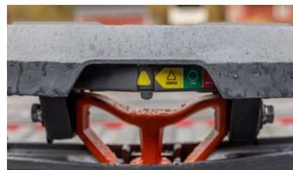
Three-position coupling indicator clearly shows coupling status
