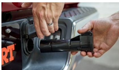
Insert Echo between the vehicle and trailer
