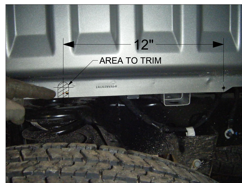
Figure 10.1: Inside Driver Side Rear Wheel Well
