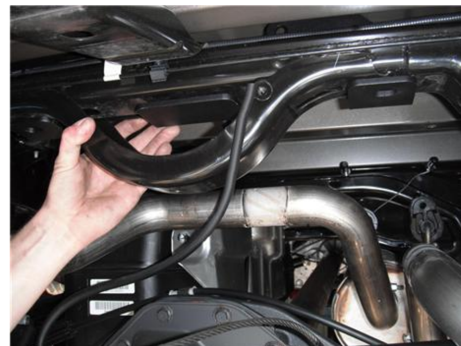
Figure 8.1: Axle Vent Hose Relocation
