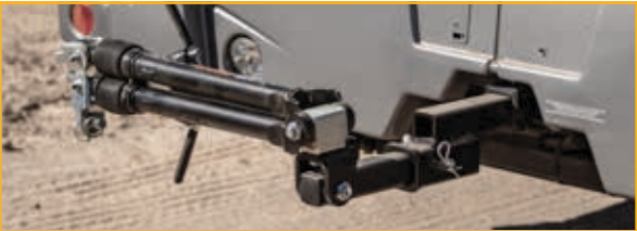
Fully sealed design and rubber sleeves protect against dirt and debris
