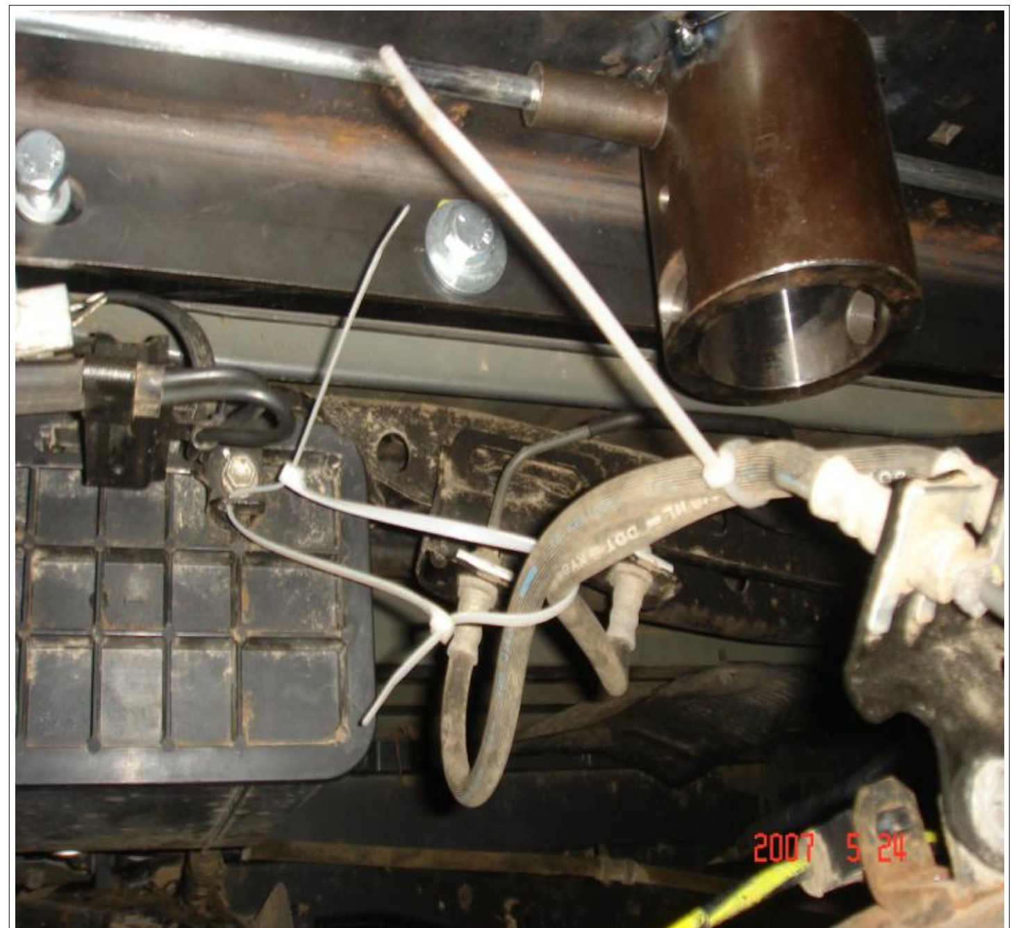
MODIFIED BRAKE LINES USING CABLE TIES
