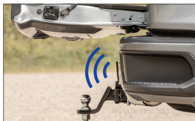
Prevents deployment of inner tailgate panel when ball mount is installed
