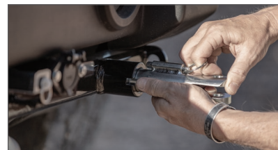
Twist-lock tabs for easy installation and removal
