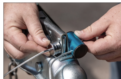
Lasso lock can be used to lock the coupler latch while towing
