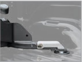
Step 2 - Close and secure the anchor levers in place
