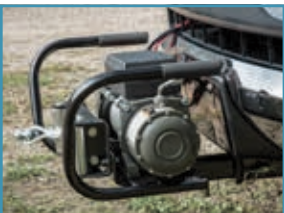
Winch mount for convenient hitch attachment as needed
