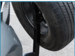
Spare tire mount with versatile 24" height to accept multiple tire sizes
