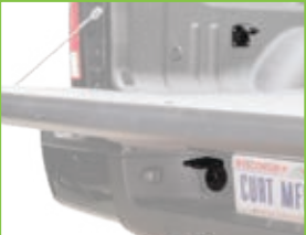
Routes a 7-way socket into rear of the truck bed (7' & 10' options available)
