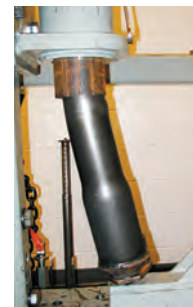
Competitor's 25K gooseneck fails longitudinal test at 11,500 lbs.
