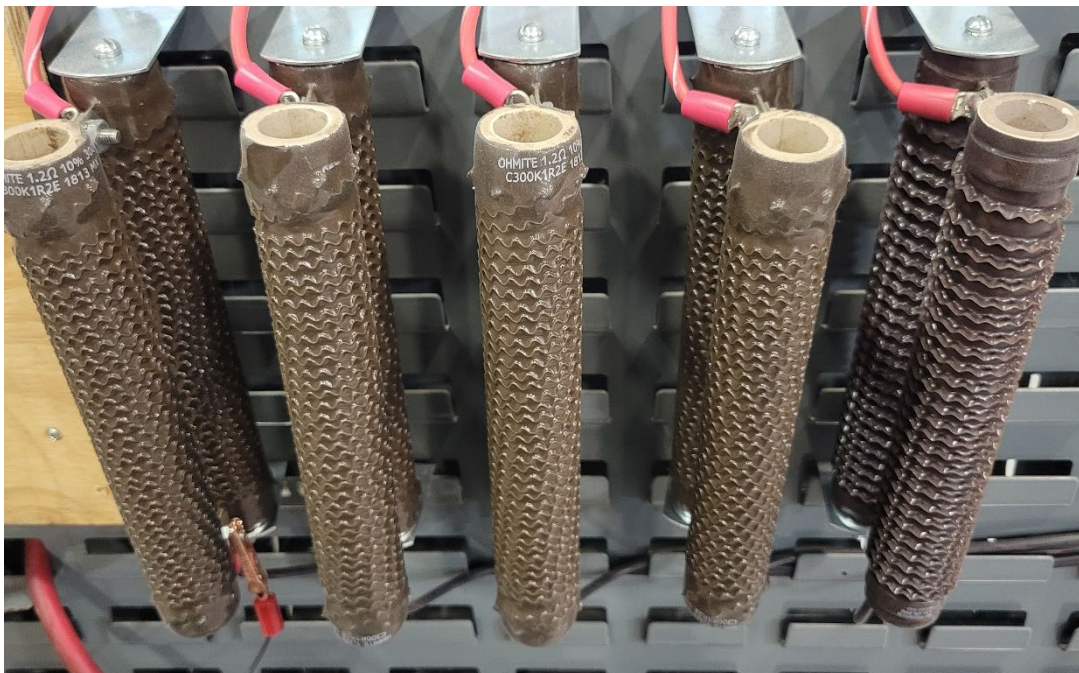
Resistive Load Bank
