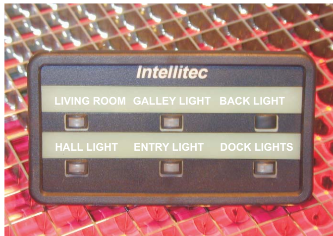
Switch Legends printed on paper with computer printer. Paper placed under overlay w/clear windows. Size 2-5/8 x 4-3/4
