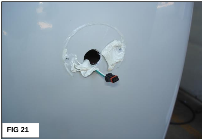
12 Fig 21: Clean the caulking from around the pod location using isopropyl alcohol and a clean rag. Wrap electrical tape around the connector, and push it into the hole, it will not be re-used.
