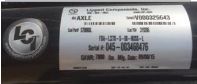
Axle Tag: Located on axle beam
