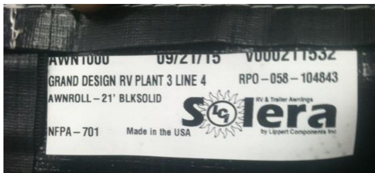
Awning Tag: When facing the coach, the tag is to the right side sewn into the seam up against the coach.
