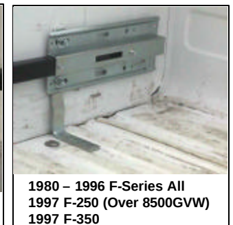
Drill in line with center of bed bolt. (Same distance from front wall)
