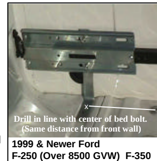
Drill in approximately center of slot, mid way between spot welds in bed floor.
