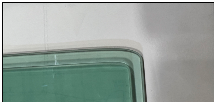
An overlay of a properly ground 6mm radius on top of a rounded or dipped corner
