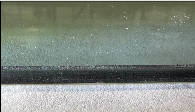
Glass with an SAE #1 ground edge viewed without magnification.
