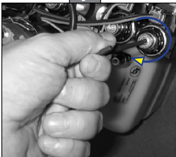
Clockwise for manual override
