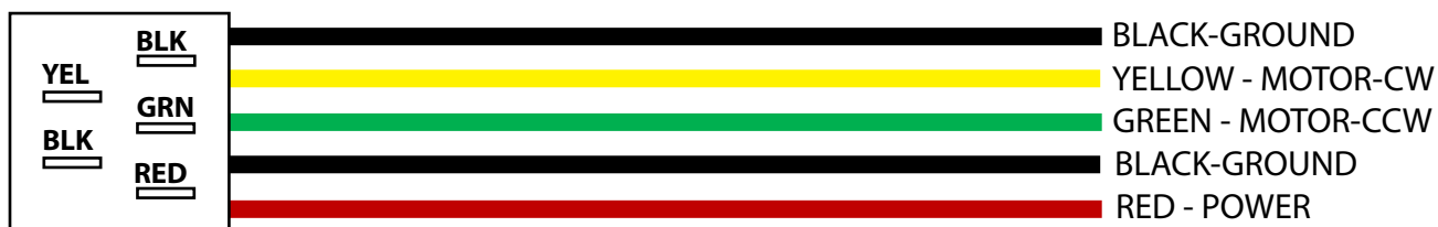
Fig. 2.2 New Slide-out Switch Kit Color Coding
