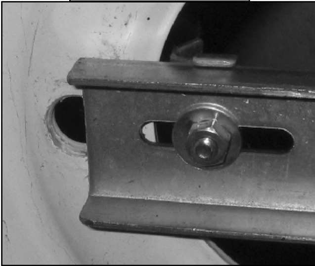
Fig. 3 - Correct ( \frac{1}{8} " Max)
