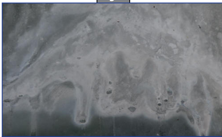
Magnified corrosion from Sodium Hydroxide on glass surface
