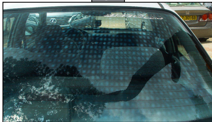
Strain Pattern visible in Passenger Vehicle Backlite
