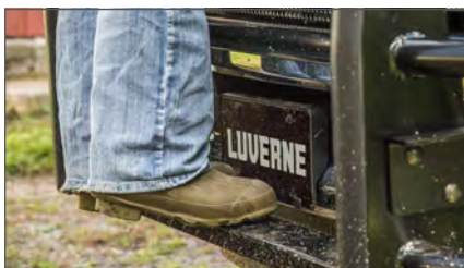
Built-in 4" diamond tread step for easy access under the hood
