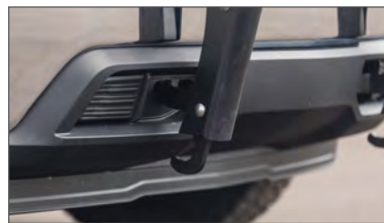
Frame-mounted uprights for improved rigidity and structural support
