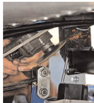
For our installation, we had to grind notches in the spring hanger in order for the crossmember bolts to fit properly.
