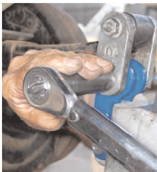
It's absolutely necessary to make sure all bolts are torqued to the manufacturer-recommended settings.
