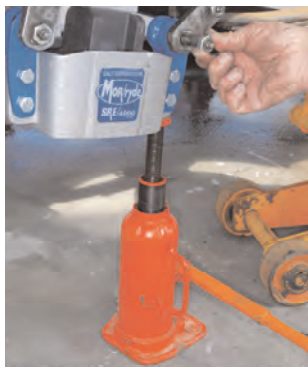
Use a hydraulic bottle jack to raise or lower the SRE to properly align the bolt holes.
