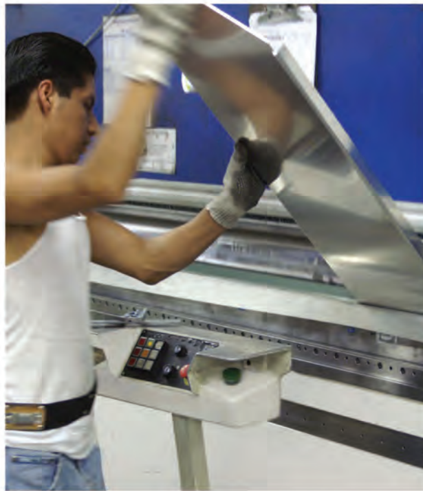
A MOR/ryde press brake operator bending a suspension part.
