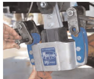
Install the new SRE equalizer with the new upper bolt and existing links (replace if worn); grease bolts prior to insertion.
