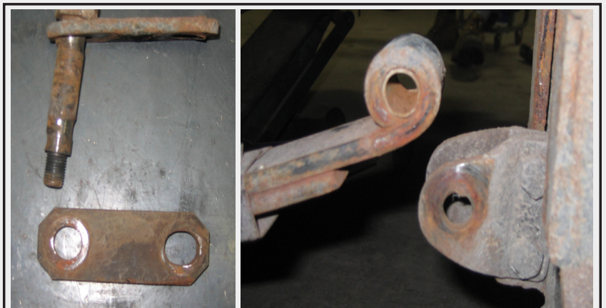
Old shackle assembly and disassembled equalizer.
