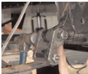
Depending on rust, the bolts holding the suspension and/or links may need to be jarred loose with a hammer.
