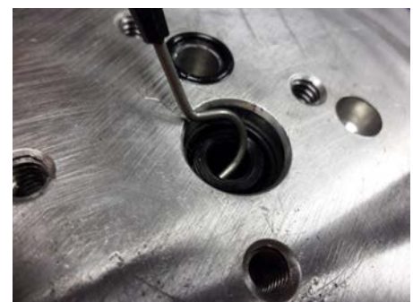
Figure 19 Removing the seal
