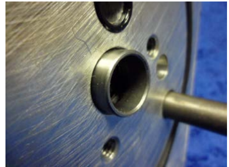
Figure 22 Insert metal spacer over new seal
