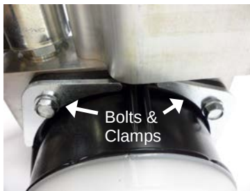
Figure 15 Bolts and clamps (4) on tank flange
