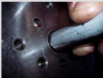
Figure 10 Setting seal in place
