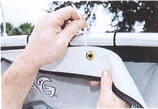
CENTER AND SECURE THE FRONT PANEL ZIPPER STRIP TO THE FRONT OF THE T-TOP COVER FRAME
