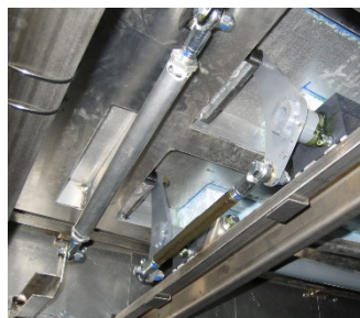
Flat-floor support and lifting mechanism
