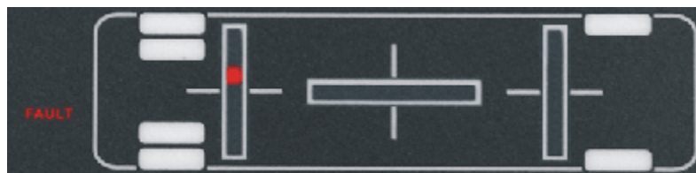
2. Short circuit in rear left Travel valve
