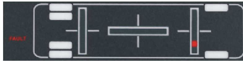
3. Short circuit in front right Lower valve
