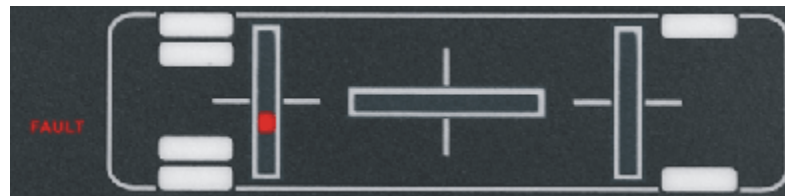
4. Short circuit in rear right Raise valve
