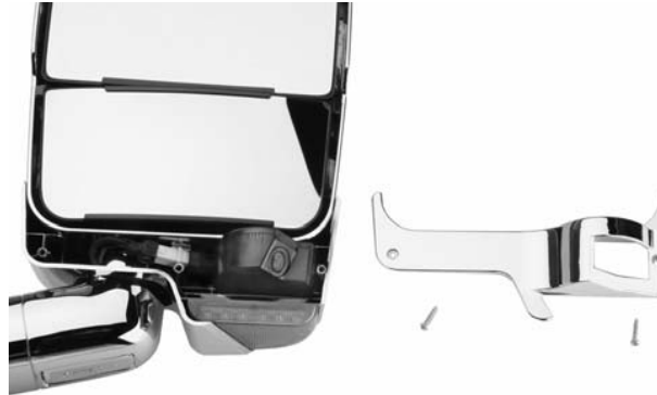
LEM with Cover plate removed
