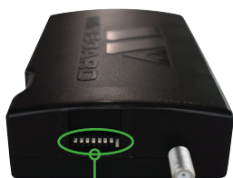
Power Inserter switches
