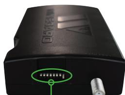
Power Inserter switches
